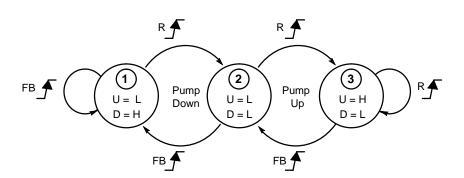
Figure 2. Phase Detector Logic Model
