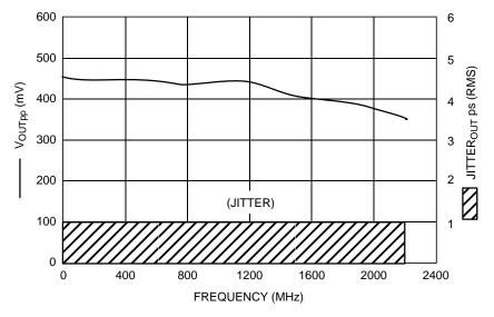
Figure 4. F<sub>max</sub>/Jitter
