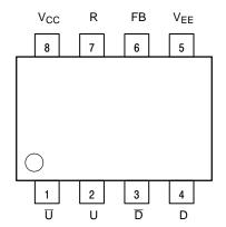
Figure 1. 8-Lead Pinout (Top View)
